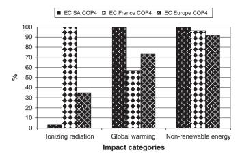
**Fig. 9.** LCA comparison for EC without heat integration in three different geographical contexts: South Africa (SA), Europe as average and France in particular.
