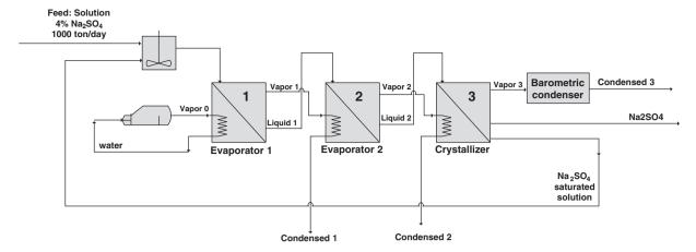
Fig. 3. Detailed flowsheet diagram considered for EC. For the sake of clarity, the freezing process to convert part of the condensed streams into ice is not shown here, but it is considered for LCA calculations.
