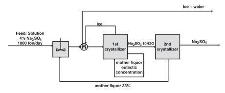
Fig. 2. Detailed flowsheet diagram considered for EFC.
