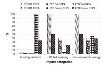
**Fig. 8.** LCA comparison of scenarios with heat integration in three different geographical contexts: South Africa (SA), Europe as average and France in particular. Different COP (coefficient of performance) values for the refrigeration of crystallizer-1 have been considered.
