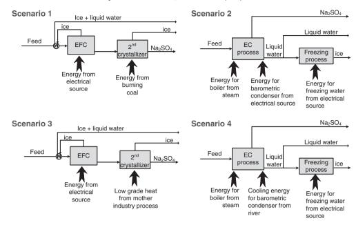
Fig. 4. Block diagrams representing the different scenarios described in Table 1. The thick arrows represent energy inputs.
