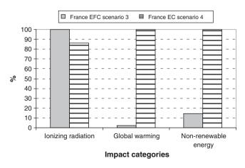
Fig. 6. LCA comparison of scenarios 3 and 4 shown in Table 1 for France.
