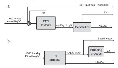
Fig. 1. Block diagrams for EFC (a) and EC (b) processes showing the boundaries for the LCA study. Both processes contain a system expansion so that the input and output products are identical.
